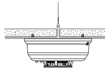
Figure 3. Mount Detector Across Ceiling Panel Support
